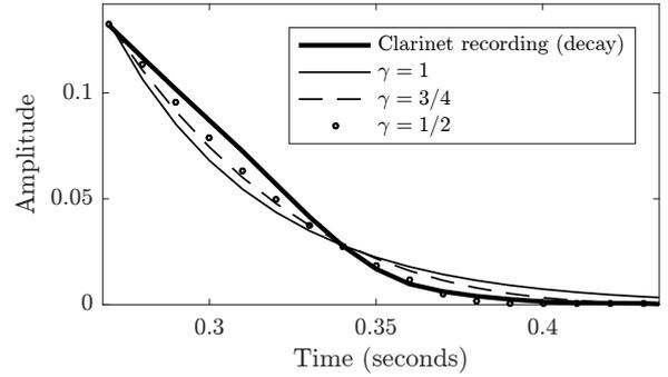
Figure 1: Comparison of amplitude model choice:  $\gamma = 1$  represents the standard model for the amplitude of a sinusoid. Selecting  $\gamma < 1$  alters the decay behaviour to more closely represent the real data obtained from the decay section of the second harmonic of a recording of a clarinet.
